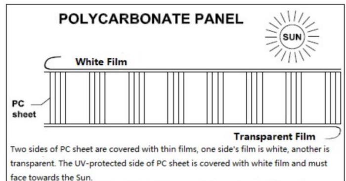
**NOTE: Some panels may have white film on both sides. These are UV treated on both sides and can be installed either way.**
