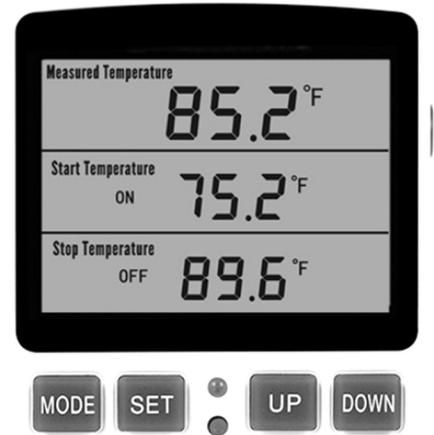
When Start/ON is set to a higher temperature than Stop/OFF, cooling mode is activated. When the OFF temperature is higher, heating mode is activated. In the example on the display above, the DT20 will cut a heater on at any temperature below 75.2 and cut the heater off when the temperature rises above 89.6.
