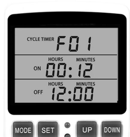
The ON setting shows how long power will be supplied to the device you have connected to the DT20. The OFF setting shows how long the device will be off in between ON times. In the example on the display to the right, power will be supplied for 12 minutes. Then it will cut the device off for 12 hours and repeat this cycle continuously.
