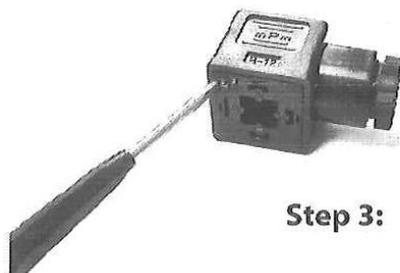
**Step 3:** Open the DIN-connector housing by using the "pry-slot"
