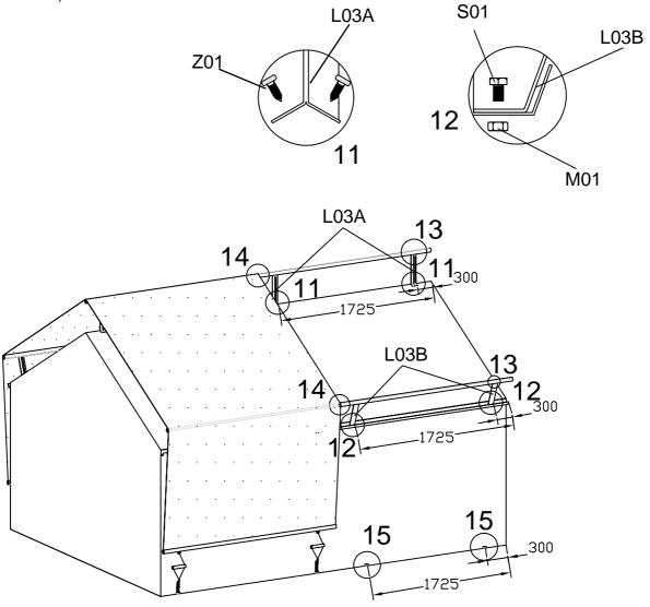
At the base of the Greenhouse place a W01 300mm from the back of the Greenhouse and place another at 1725mm. Predrill the holes using a 6mm diameter drill and screw fix the brackets in place being careful not to over tighten. Repeat the process on the opposite side of Greenhouse.
