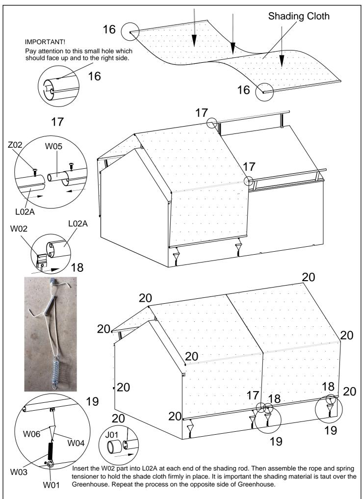
PLEASE NOTE: If your Grange Greenhouse exceeds 4mL and requires additional 2mL Shading modules the W05 joiners are not provided. It is only necessary to join each 4m section.
